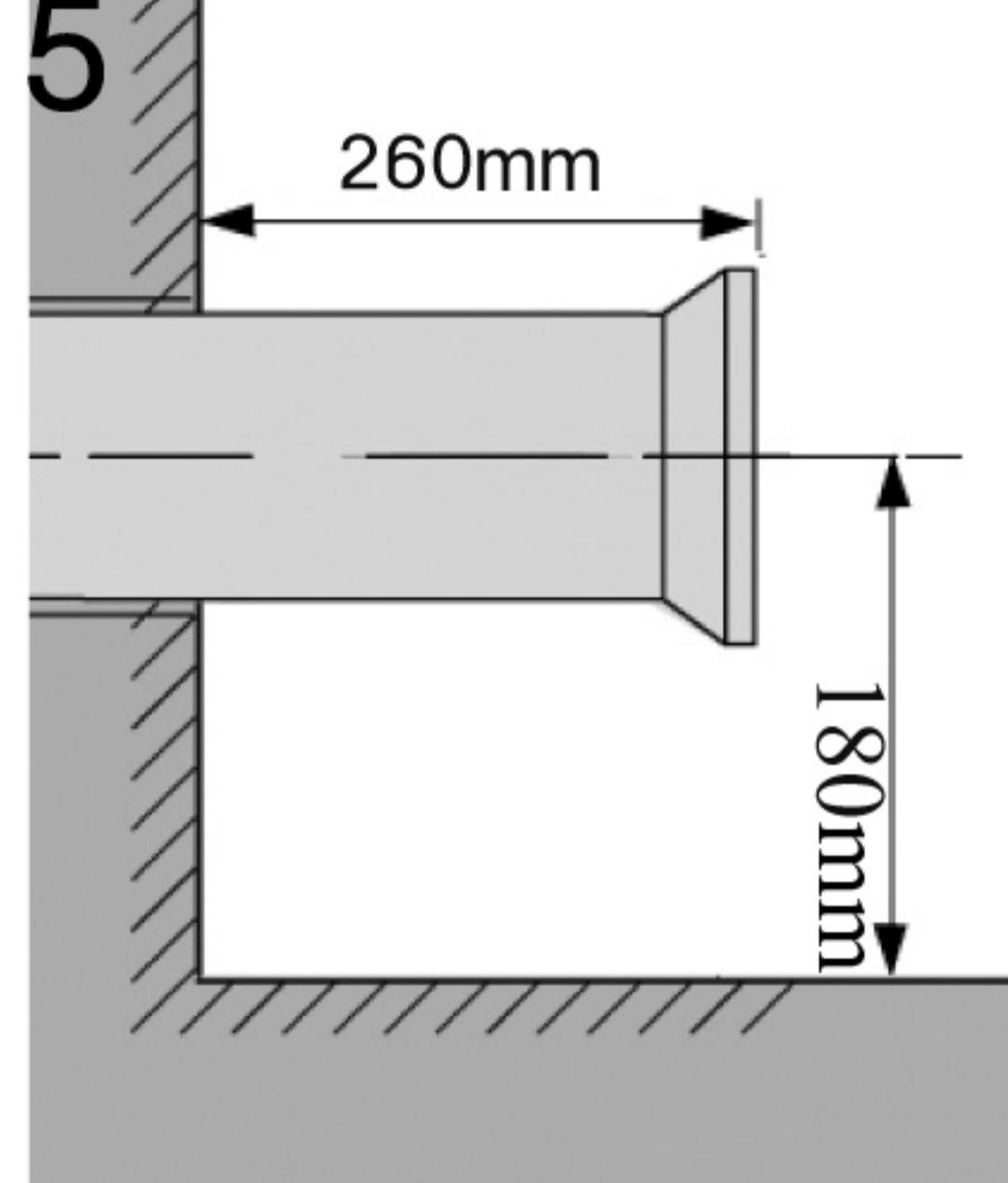
5. Set up waste pipe so that the end of the pan collar extends from the finished wall.
