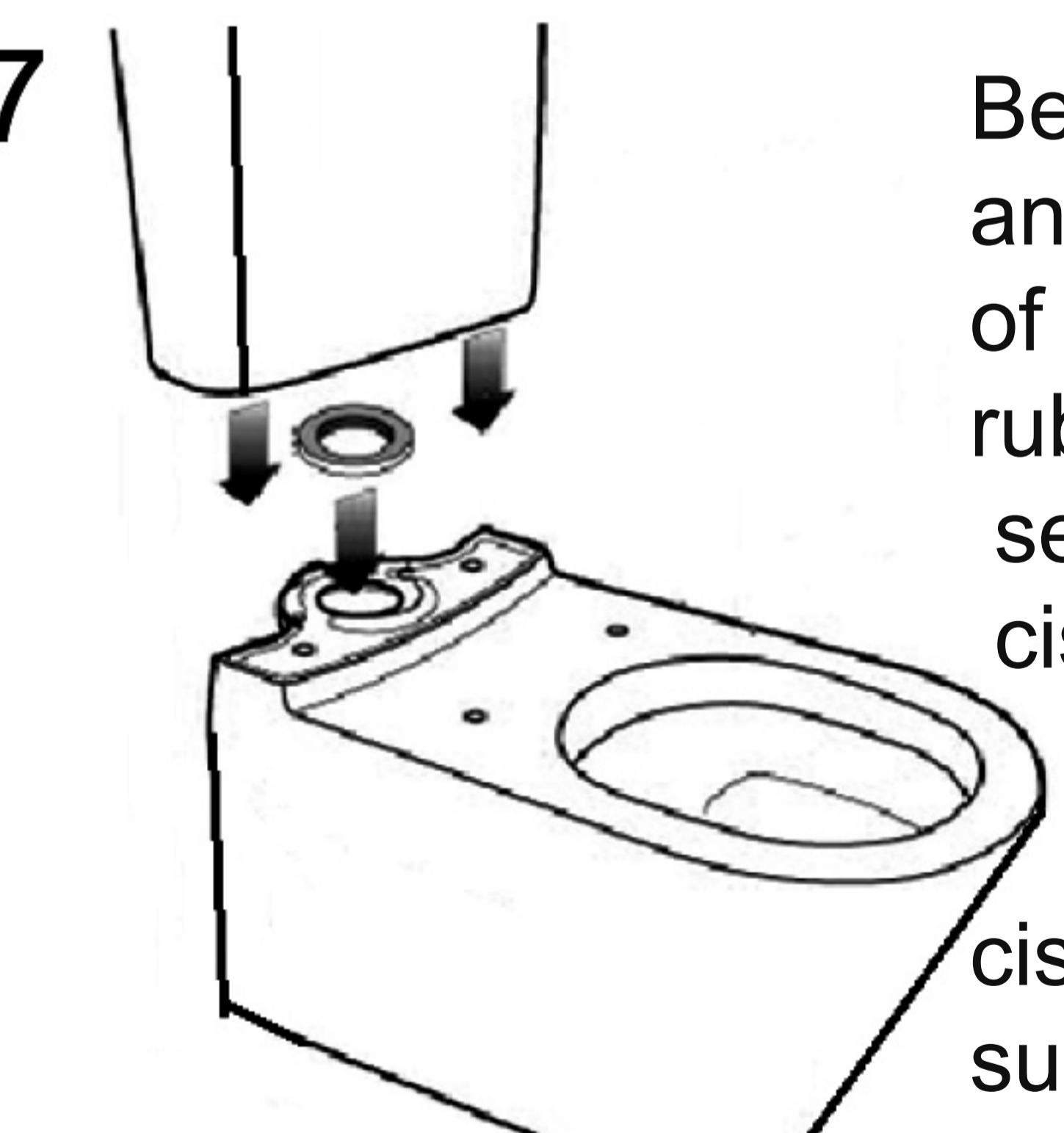
Before installing cistern, please check bungs and valves are tightened correctly. Put a bead of silicon to both upper and lower surfaces of foam rubber seal between cistern and pan. Place rubber seal at the bottom of the cistern, then gently lower cistern onto pan. Make sure the screws holes are matching between cistern and pan. Apply a beat of silicon around the bolts, then secure cistern to the pan. Before tightened fully make sure cistern sites square and straight to pan.
