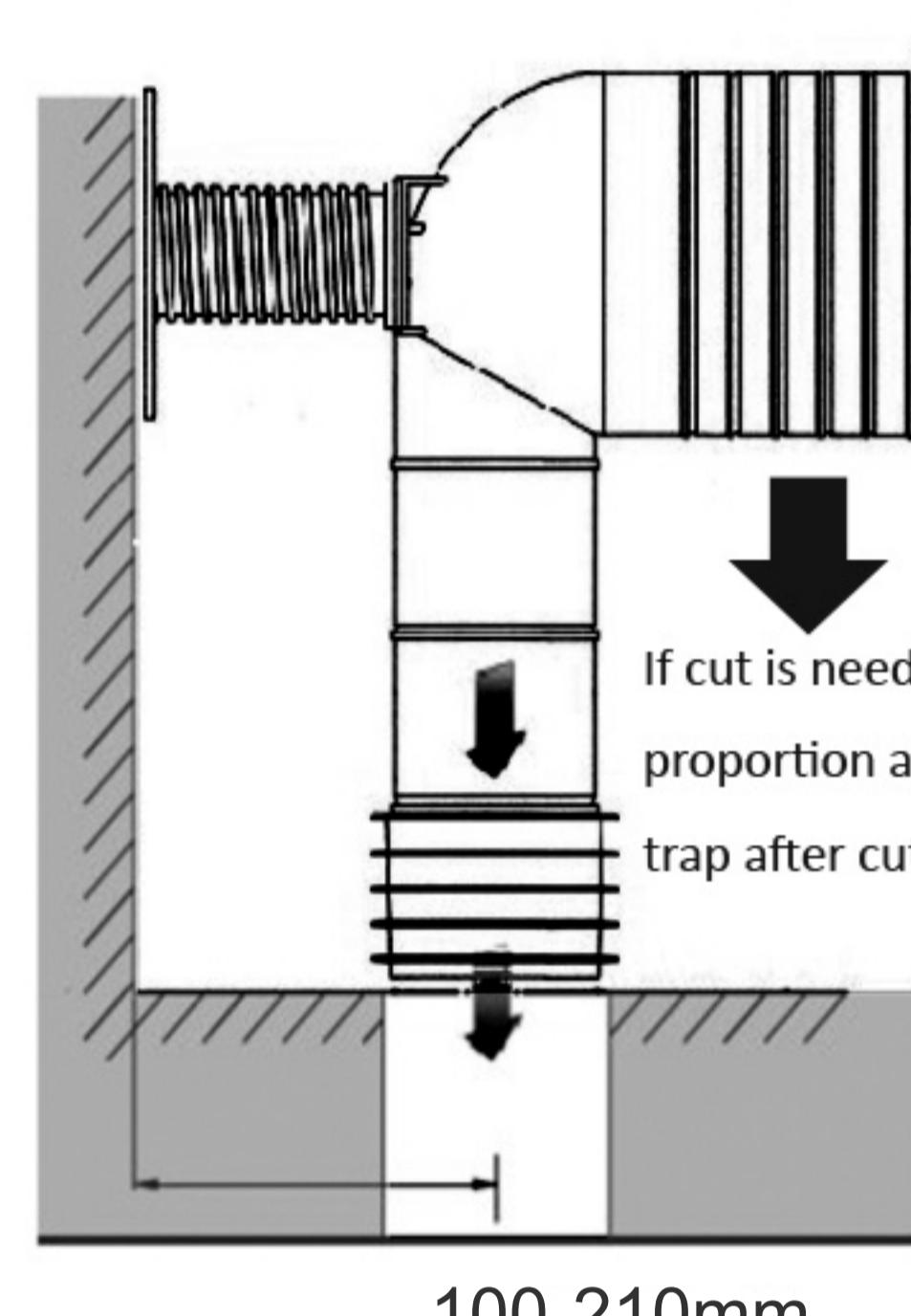
2. Lubricate the fins of the pan bend and position into waste pipe.
