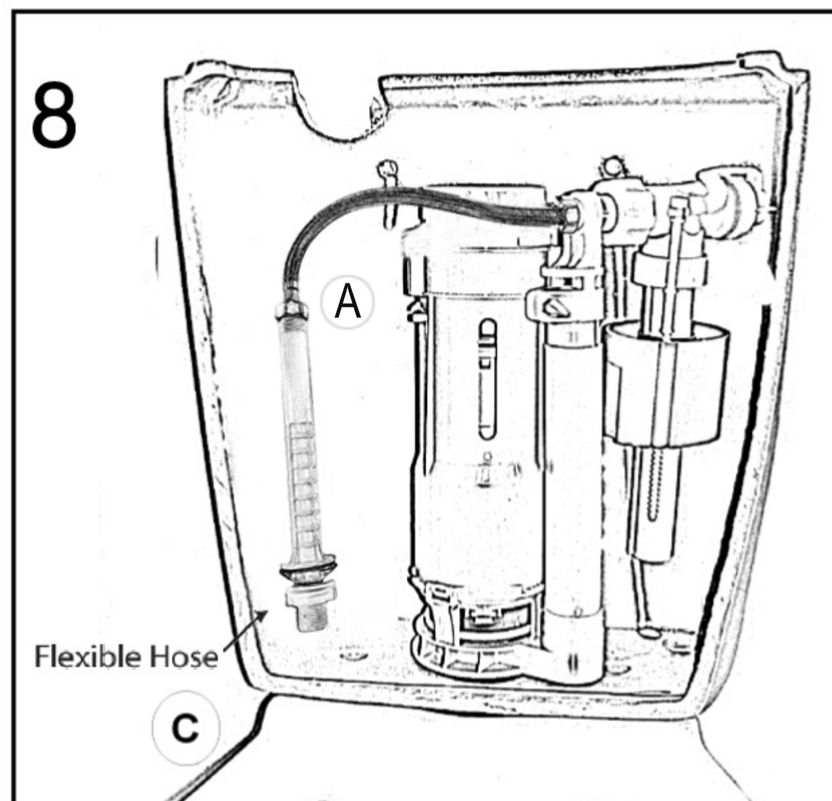
8. IF BACK INLET, SKIP THIS STEP. For Bottom(left hand) inlet connection, please connect flexible hose to plastic tube A, then complete stop tap connection to underside of cistern plug C. Fill cistern and ensure correct water level. Note: Inlet valve can be adjusted if required.
